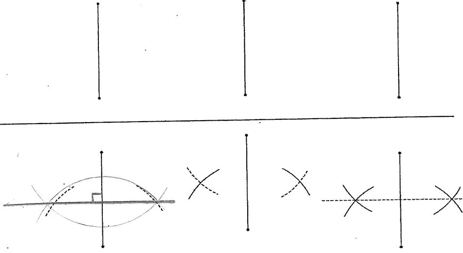
Step 2 Put the point of the compass on one end of the segment and construct an arc above and below the segment.
