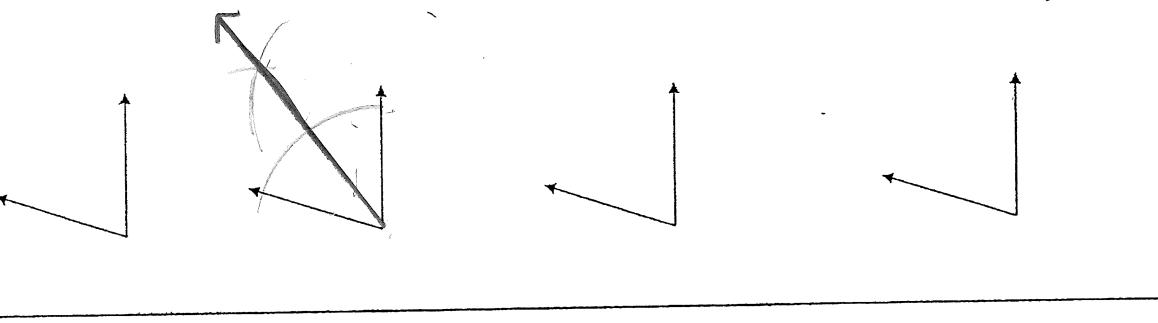
Step 2 – Construct an arc crossing both sides of the angle. Put the point of the compass on the vertex of the angle.
