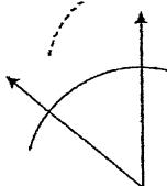
Step 3 – Without changing the compass measure from step 2, put the point of the compass on one side of the angle where the arc crosses it. Then draw an arc on the interior of the angle.
