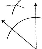
Step 4 – Draw the angle bisector by connecting the vertex of the angle with the point where the two arcs from steps 2 and 3 cross.
