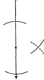
Step 5 – Draw a segment connecting the intersection of the arcs and the given point.
