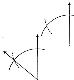
Step 6 – Draw the second side of the angle by connecting the endpoint of the ray (your vertex) with the point where the two arcs intersect.
